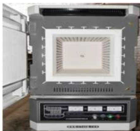
Figure:3. Temperature-controlled electric furnace.
